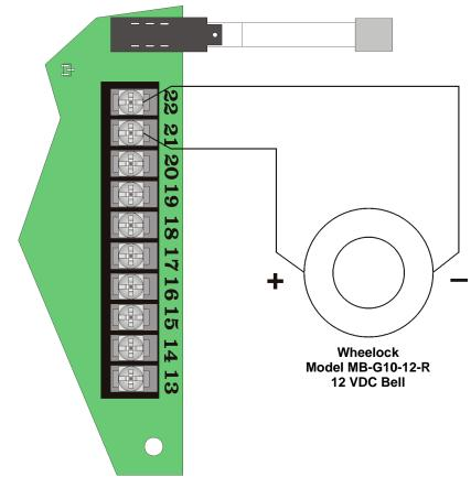
Figure 3-13 illustrates how to wire a non-supervised notification device to the control panel.
