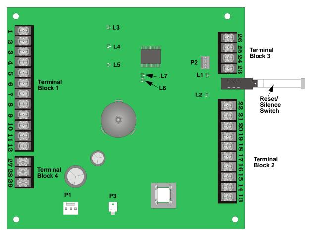
Figure 3-2 5104 Circuit Board
