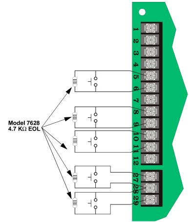
Figure 3-9 Model 5104B Class B (Style B) Loops
