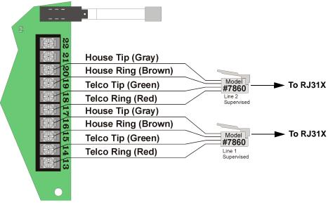
Figure 3-15 Telephone Line Connections
