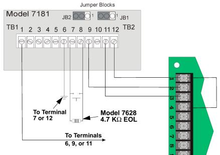
Figure 3-11 5104 Class A Panel Configuration to a 7181 Class B Sensor
