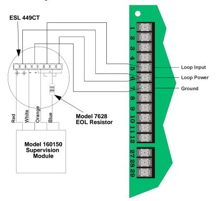
Figure 3-10 4-wire Smoke Detector Connections
