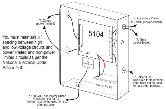
Figure 3-1 Wire Routing Example
