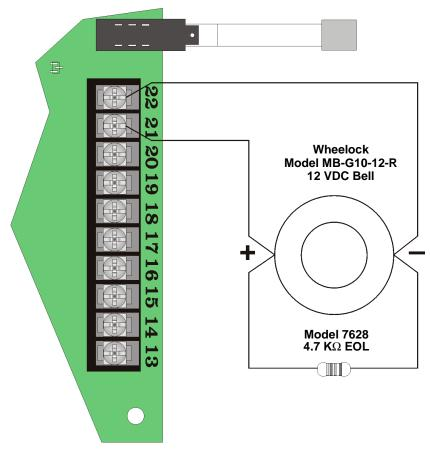
Figure 3-14 Supervised Alarm Bell Wiring
