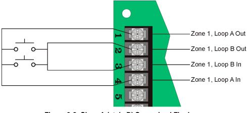
Figure 3-8 Class A (style D) Supervised Fire Loop (Normally Open Sensors Only)
