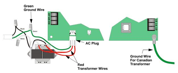
Figure 3-3 AC Transformer Connections
