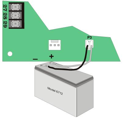
Figure 3-7 Backup Battery Connections
